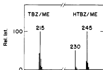
Figure 1. Partial mass spectra of on-column methylation products of TBZ and HTBZ.
